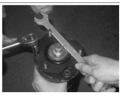
\*\* Caution: Use the factory nuts with the factory studs\*\*10. Run down nuts snug with end wrench. Torque to OEM specs.
